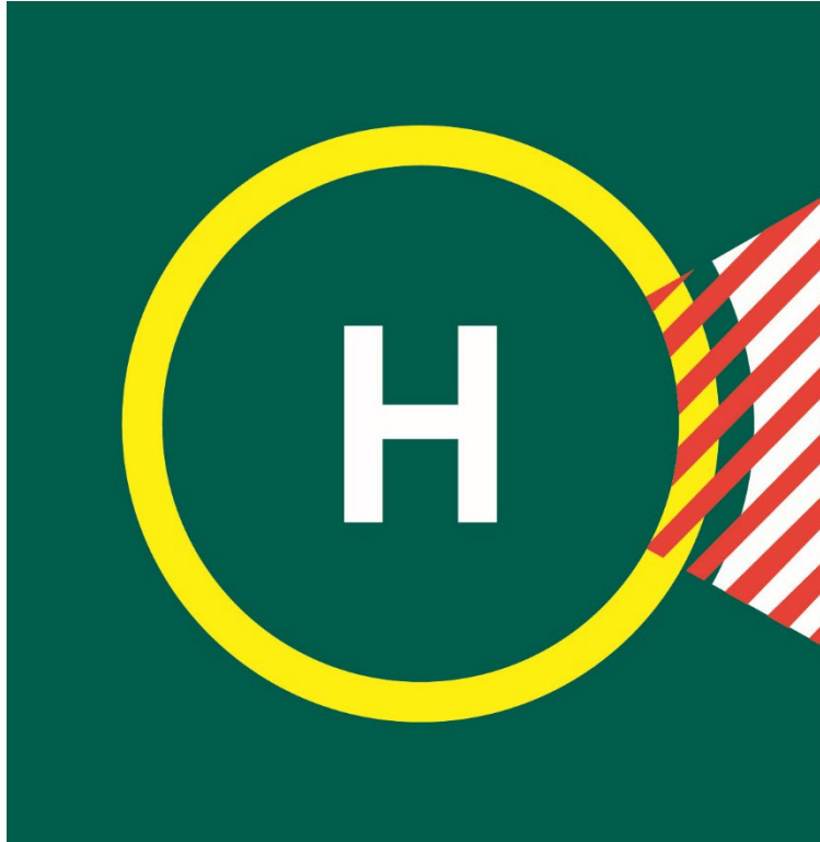
Figure 6: Example of prohibited landing heading marking
